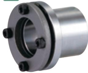
Compared to the mechanical connecting element, the number of bolts can be reduced and attachment and detachment can be simplified. The concentricity is 0.05 mm so mounting can be performed with relatively high precision.
