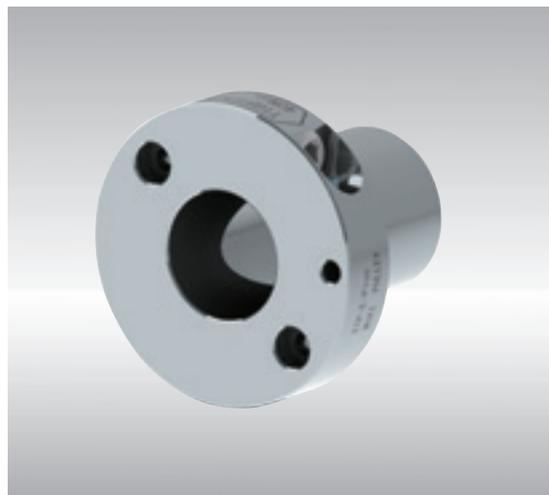
Additional processing is possible to make a counterbore or tap to allow ETP positioning when installing on equipment. (Limitations apply to processing locations; contact Miki Pulley.)
