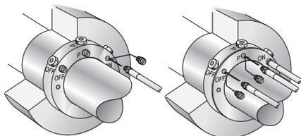
If the return hose is not connected to the ON port, the oil inside may spew out.
