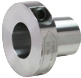
The shaft and the hub can be connected easily and quickly with 1 bolt. Since the concentricity is as accurate as 0.02 mm, this model is most suitable for applications that require high accuracy and where the device is frequently attached and detached. It is structured to be tightened from the radial direction to save work space.
