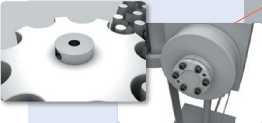
ETP bushing is used to match the phase of the alignment table with the phase of the alignment screw.
