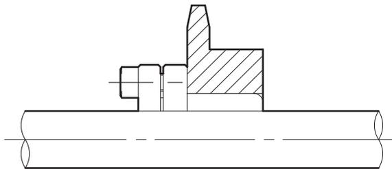
Drilling a Stepped Hole in the Hub for Connection
