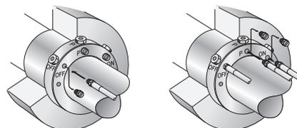
Never apply pressure before the ETP-HYLOC is mounted to the shaft and hub.
