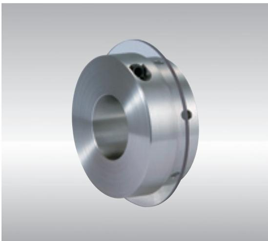
This is a hydraulic slitter knife holder. This holder is used to position the rotating knife to cut tin, iron, aluminum plates, or paper sheet in any position. Positioning in the shaft direction can be performed arbitrarily with 1 bolt. For the angular deflection caused by detachment and attachment, a micron meter ( $\mu\text{m}$ ) level repeatable accuracy can be maintained.
