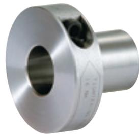
The shaft and the hub can be connected easily and quickly with 1 bolt. Since the concentricity is as accurate as 0.006 mm, this model is most suitable for applications that require high accuracy and where the device is frequently attached and detached. It is structured to be tightened from the radial direction to save work space.
