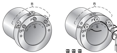
Then, mount the ETP-HYLOC to the shaft and hub.
