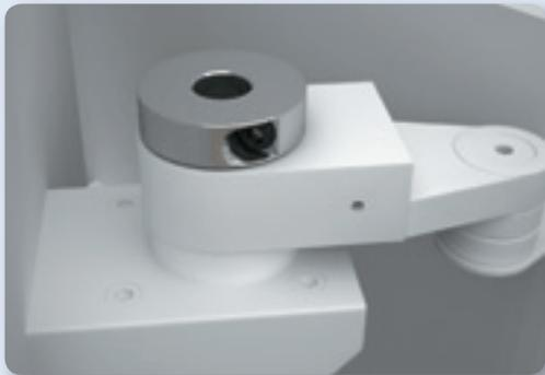
ETP bushing is used to connect the mold fixing shaft and the shaft of the index feeding unit. Connection with one bolt substantially reduces the adjustment time.
