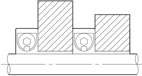
Connection with a Roller of a Printing Machinery
